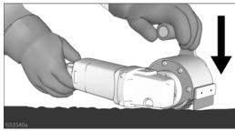
2. When ready to stop cutting material, lift the cutters off of the surface, release the trigger, and allow the cutters to come to a stop.
