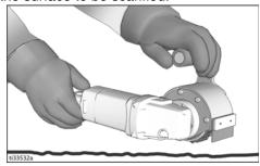
4. Depress the trigger and adjust the speed dial to the desired setting.
