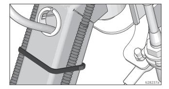
8. Attached laser to desired location on gun arm.
