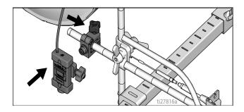
9. Route switch wires down to battery and connect to the (+) and (-) terminals, and route jumper through gun cable hole.
