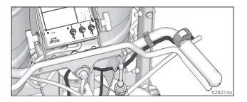
5. Route switch wiring between piston and square tube, and down to battery.
