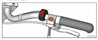
3. Attach laser to desired location on the gun arm.
